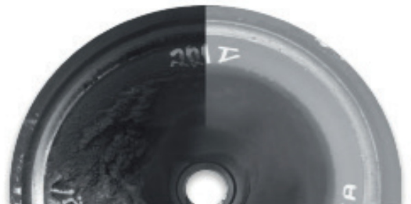
Figure 1: Impact on exhaust valve seat with slide fuel valve before and after retrofitting
