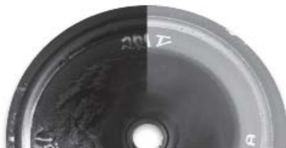
Impact on exhaust valve seat with slide fuel valve before and after retrofitting
