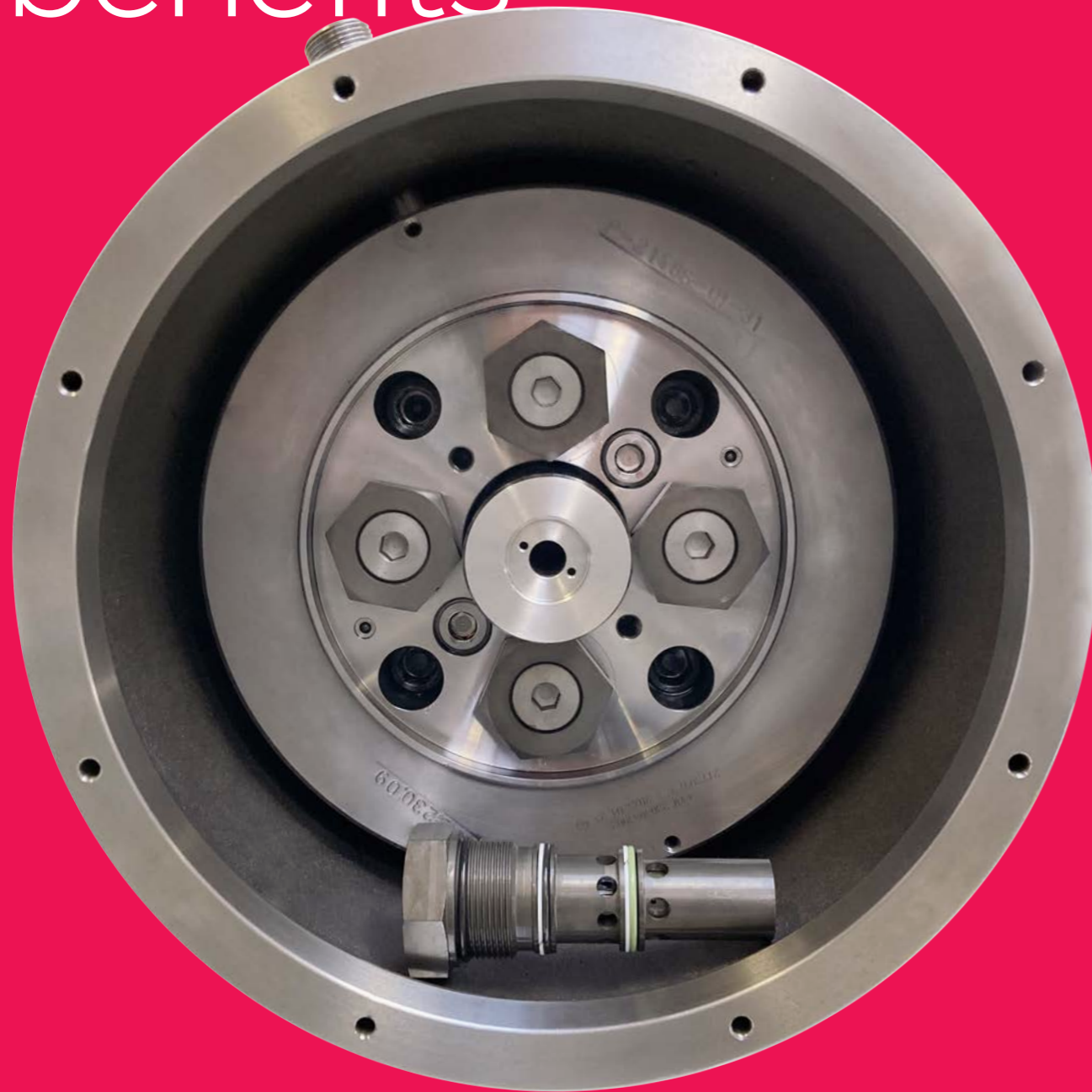
ODG (Oil Distribution Gear) unit with POCVs (Pilot Operated Check Valves)
