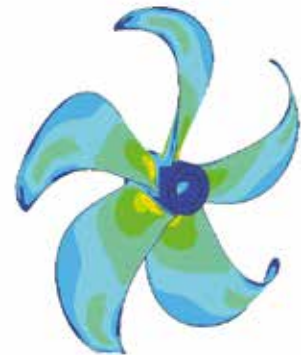
Blade roots Von Mises stresses in wake field, normal loading
