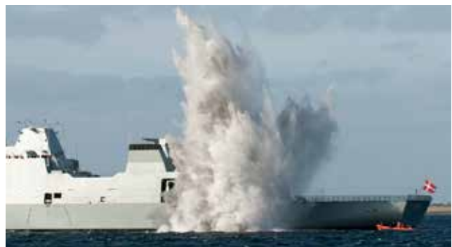
Full-scale shock testing – from underwater explosion
