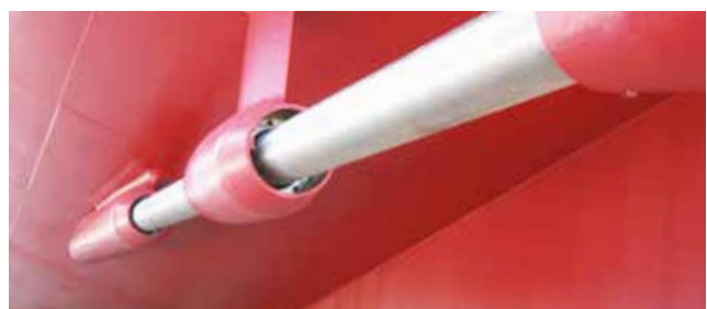
Shafting: Struts, bearings and an Inconel clad-welded tail shaft
