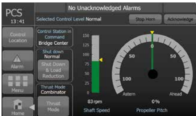
Fig. 11a: Home screen – single CP propeller plant
