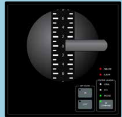
Fig. 7: Single-handle version - MHP - for CPP
