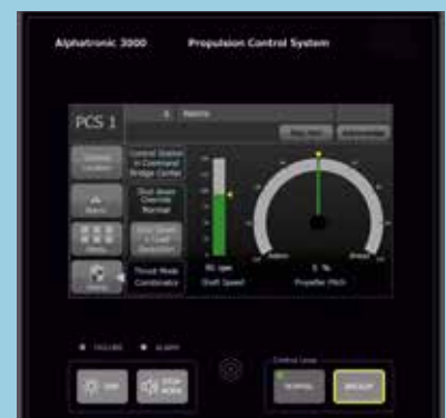
Fig. 10: Propulsion Control Panel - PCP - for CPP
