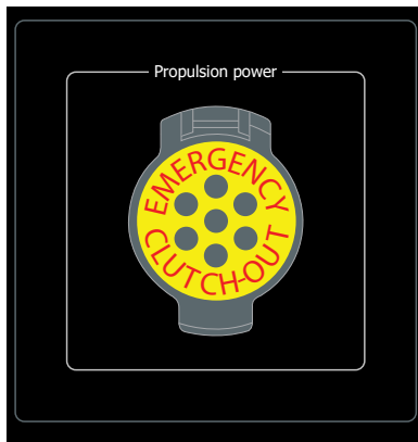
Fig. 25: Emergency Clutch-out Panel – ECP
