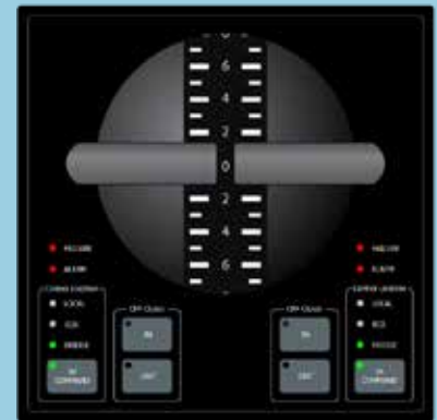
Fig. 8: Double-handle version - MHP - for CPP
