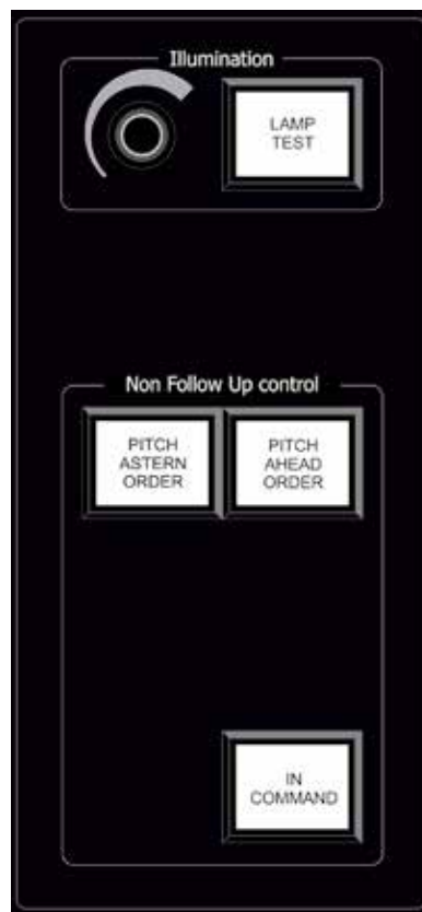
Fig. 26: Non Follow Up control panel – NFU
