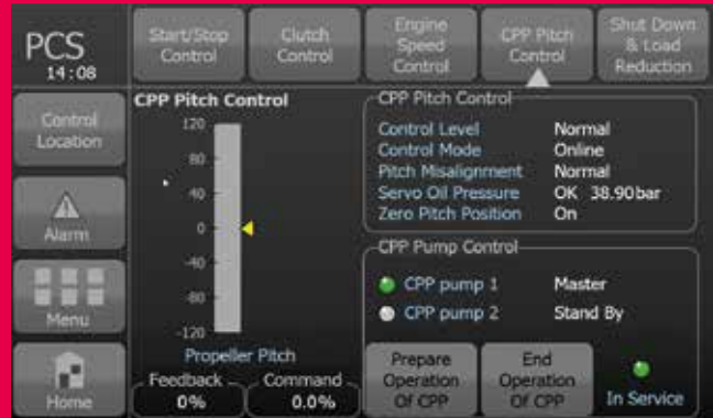
Fig. 18: CPP Pitch Control
